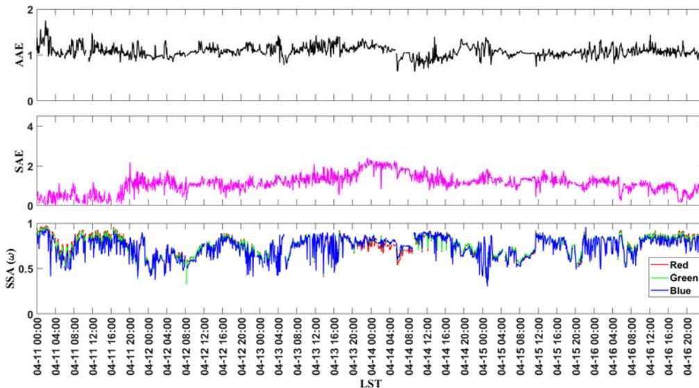
**Figure 2.** Example of AAE, SAE, and SSA calculated from optical TAP and nephelometer measurements from the BC<sup>2</sup> El Paso site. AAE, SAE, and SSA profile for blue, red, and green wavelengths with 5 min averages from April 11 to 16.
