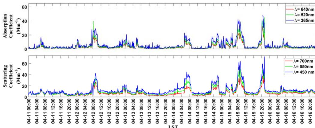
**Figure 1.** Example of particle-based optical measurements using the *Tricolor* Absorption Photometer (TAP, top) and nephelometer (i.e. scattering, bottom) from the BC<sup>2</sup> El Paso site. Absorption and scattering profile (5 min averages) of blue, red, and green wavelengths from April 11 to 16.
